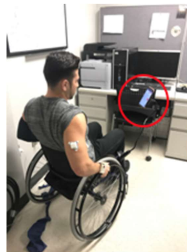
Figure 3: Phone Suspended in Front of User on Portable Stand Attached to Wheelchair
